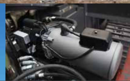
Electric pre-heating system Engine start below -50°C temperature Engine coolant hiting system by diesel fuel Webasto installed
