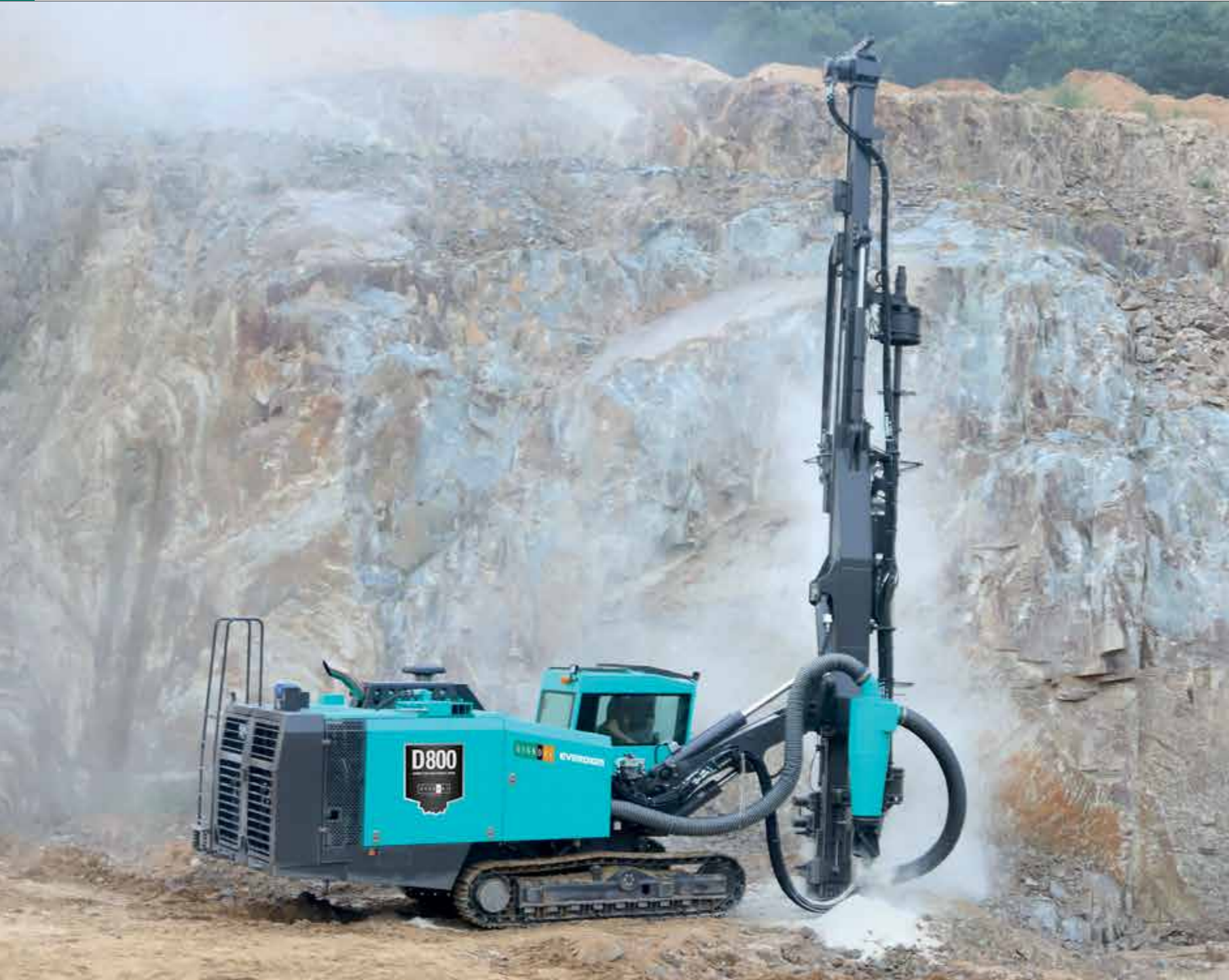
Hydraulic rotation unit ERD65 - Max RPM 53 RPM, Max Torque 5,700 Nm
