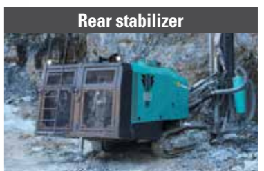
Rear stabilizer To support machine for better straightness of drilling hole and maintenance
