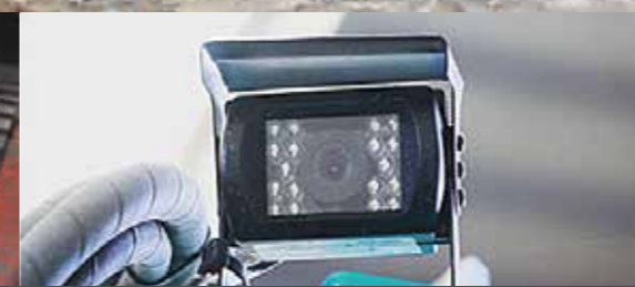
Rear view camera To check an object on the rear side for safety
