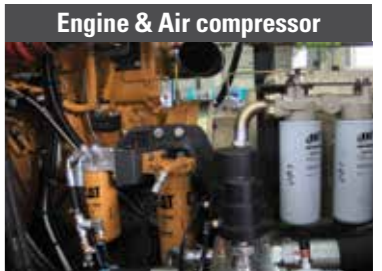
Engine & Air compressor - CAT C15 Tier3 Engine Installed - Pump-Engine-Comp. Direct mounting -> Minimize loss of engine power - Compressor : GHH (Germany)
