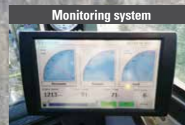
Monitoring system - Engine condition monitoring - Compressor condition monitoring - Drilling pressures display - Failure log recording, Mast X-Y angle
