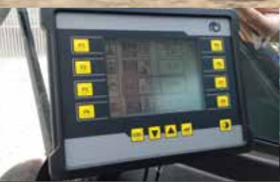
Drilling depth & Angle indicator Efficient drilling support
