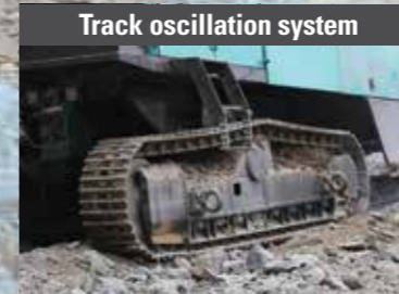
Track oscillation system Independent oscillation - Angle 20° (F10° / 10°) - Easy movement on rugged ground condition
