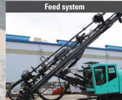
Feed system Feed cylinder + Rope system - Feed force, max 8,992 lbf (40 kN) - Tractive pull, max 11,240 lbf (50 kN)
