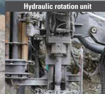
Hydraulic rotation unit ERD65 - Max RPM 53 RPM, Max Torque 5,700 Nm
