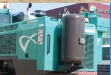
Water misting system Prevent hole crumbling and bit jamming during drilling
