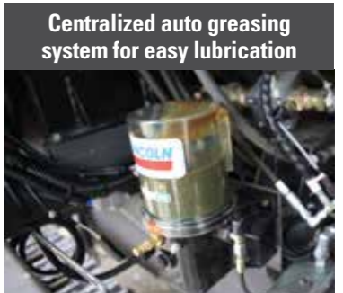
Centralized auto greasing system for easy lubrication
