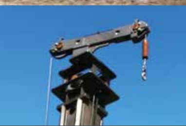
Hydraulic winch Handling and lifting tube for installing and removing from ARC
