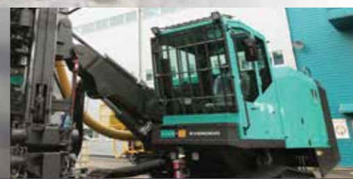
Safety guard Protecting cabin glass from relatively bigger flying object
